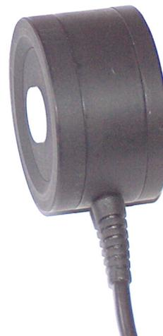
Measure probe **G.PAR-100** make complete photometer including:
