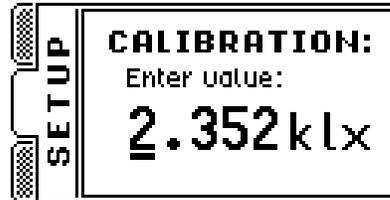
Value editing is allowed by inputting values from alphanumeric keyboard. Position of cursor can be changed by key **▶**. Keys **▼▲** change multiplication factor of unit. Approving reference value can be made by key „Calibration” available through hole in left lateral of steer unit (Illustration 1.). If inputted value does not fit instrument criteria, meter will generate one of following error communicates:
