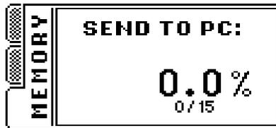
Transmission will start after pressing keyboard key ◀↵. In lcd display user may see overall progress of memory transmission. Transmission process can be broken through keyboard key
