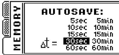
Time values change is done by key's ▲▼▶ and approve by key ◀↵, after that new window with allow user to edit comment will appear. In this window user make default comment that instrument will give for all cell's during auto save option enabled :
