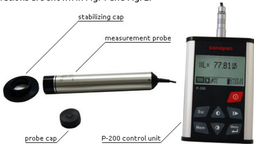
Fig. 1. Configuration of the LMC-10 measurement probe with the P-200 control panel.
