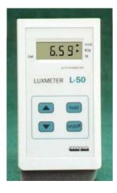
Reading of measured value is done on the LCD, directly in lux or kilolux. Exceeding the measuring range (overload) is indicated by one on the first digit and extinguishing of remaining digits.
