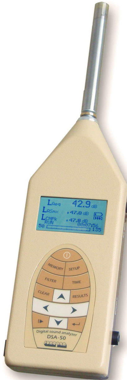
Fig. 1.1. DSA-50 digital sound analyzer – general view.
