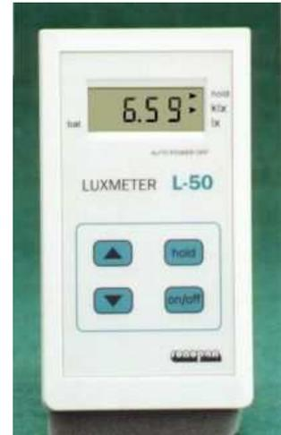
Reading of measured value is done on the LCD, directly in lux or kilolux. Exceeding the measuring range (overload) is indicated by one on the first digit and extinguishing of remaining digits.
