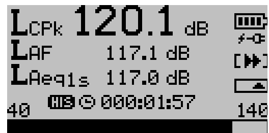
Fig. 3.6. Results screen 3 – measurement history log registration turned on.
