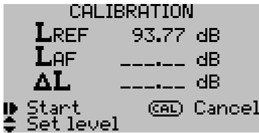
Fig. 3.17. Calibration – setting reference level.
