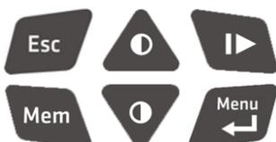
In order to switch the instrument on, press the following key:
